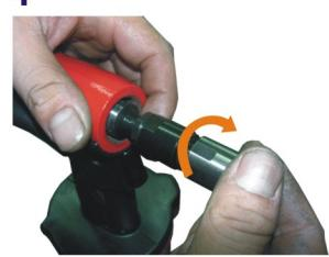
Place Jaws ⑯ into the Jaw Housing ⑯ after apply thin layer of lubricant on the inner surface. Then, fasten the Jaw Housing ⑯ and Jaws ⑯
