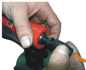
Turn the Jaw Housing Coupler ⑯ till against the Lock Nut ⑯
