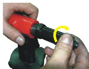
Turn the Head ⑯ into the Hydraulic Section ⑯ for 2 ~ 3 turns.
