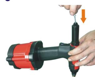
Hold the tool and keep the Head ⑯ vertically upward. Then, insert the mandrel of blind rivets into the Nosepiece ⑯ while keep turning down the Head ⑯ until the mandrel drop to the bottom.
