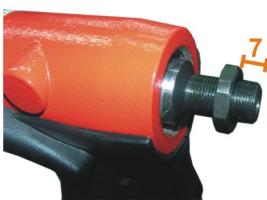
Turn the Lock Nut ⑯ through the threads of the Hydraulic Plunger ④ until 7 threads left.
