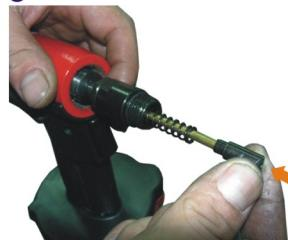
Insert the Jaw Pusher Spring ⑯ and Jaw Pusher ⑯ or (Spring ⑯ and Jaw Pusher ⑯) into the central passage of Jaw Housing Coupler ⑯
