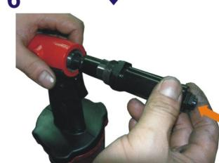
Place proper size of Nosepiece ⑯ on the Head ⑯ and screw the Nut ⑯ from the rear threaded end.
